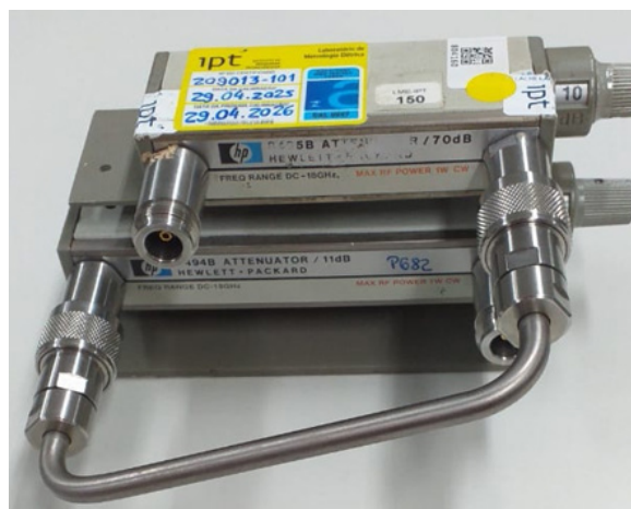
Figure 3. Calibrated step attenuator used as standard to SFRA calibration.
