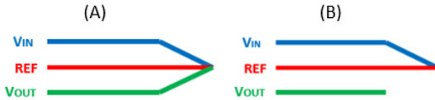
Figure 2. Checks to assess the accuracy of SFRA measurements. The VIN, REF and VOUT connectors are generally of the BNC type
