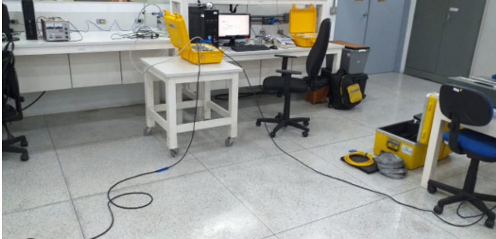
Figure 4. Calibration setup of one of the SFRA.
