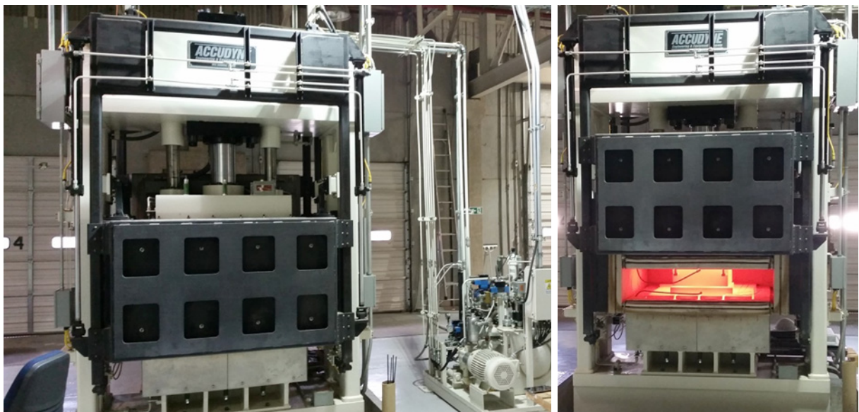
Figure 6 – Lightweight Structures Laboratory's superplastic forming Accudyne machine.
